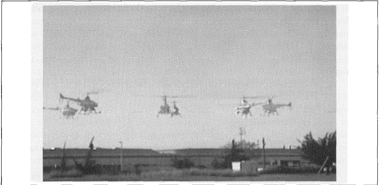
Figure 21.10 Superimposed time-lapse images of an autonomous helicopter performing a very difficult “nose-in circle” maneuver. The helicopter is under the control of a policy developed by the PEGASUS policy search algorithm. A simulator model was developed by observing the effects of various control manipulations on the real helicopter; then the algorithm was run on the simulator model overnight. A variety of controllers were developed for different maneuvers. In all cases, performance far exceeded that of an expert human pilot using remote control. (Image courtesy of Andrew Ng.)
